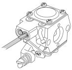
When your chain saw is equipped with a carburetter that features movement limiters, the carburetter should be adjusted according to the instructions under the heading Carburetter with movement limiters.
